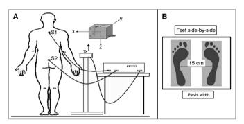
**Figure 1.** A: Location of the electromagnetic sensors. Tx: Transmitter and representation of the three planes; S1 and S2: 1st thoracic vertebrae and sacral region; B: Surface with position of the feet.
