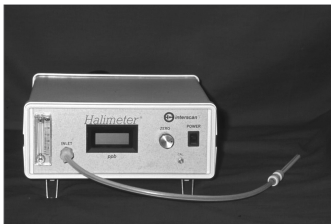
Figure 1. Halimeter: an objective measurement of Volatile Sulphur Compounds (VSC)
